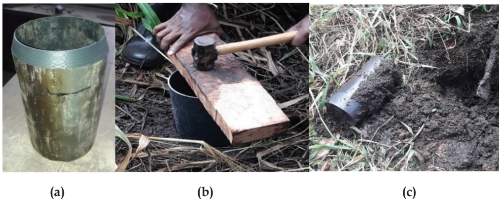
Figure 2 - Sampling tube used and the sampling procedure: (a) Tapered PVC tube; (b) PVC tube driving for sampling; (c) Sample extraction
